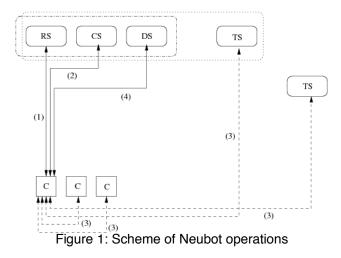
The diagram in Figure 1 shows the basic operations of the Neubot architecture. Each Neubot client (C) first registers (1) with a Registration Server (RS), which identifies the client. The RS also informs the Neubot client about the other available clients.
